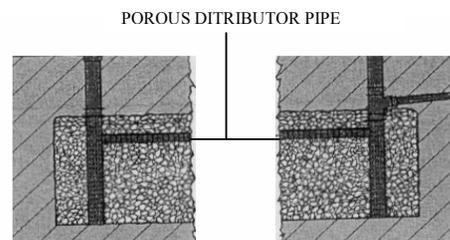
**Fig 4** Trench-type soakaway with horizontal distributor pipe
